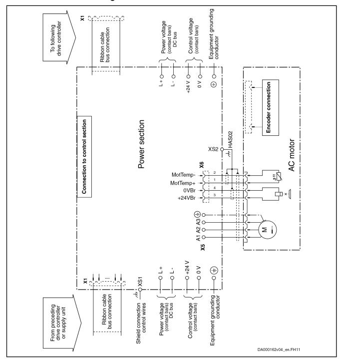
Fig. 4-1: Connection Diagram HMS
