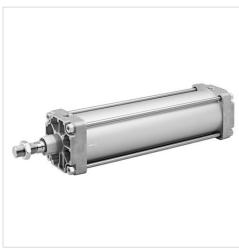
Standards ISO 15552 Certificates ATEX optional Compressed air connection Internal thread Working pressure min./max. 2 ... 10 bar -20 ... 80 °C Ambient temperature min./max. -20 ... 80 °C Medium temperature min./max. Medium Compressed air Max. particle size 50 µm 0 ... 5 mg/m<sup>3</sup> Oil content of compressed air
