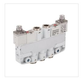
Type Spool valve Activation Electrically Pilot Internal Soft sealing Sealing principle 3 ... 7 bar Working pressure min./max. -10 ... 50 °C Ambient temperature min./max. -10 ... 50 °C Medium temperature min./max. Medium Compressed air
