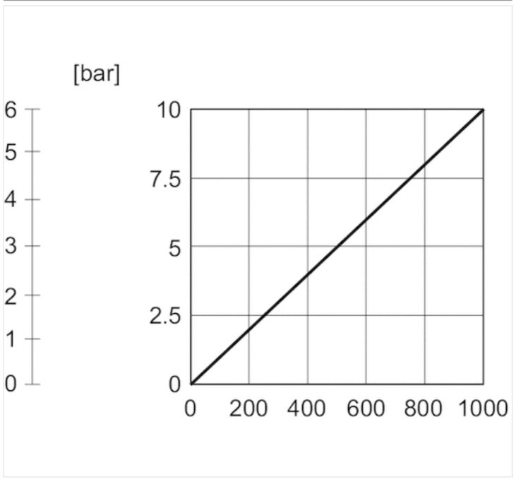
The regulator features a resolution of 10 bits (bit 0 to 9) for the serial nominal value and serial actual value: The nominal value and actual value range for the 10 bar version lies in the range of 0 to 1000 at a resolution of 10 mbar.
