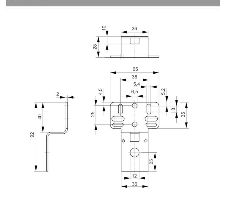
For assembly of the W01 mounting plate, the rear cover of the air preparation unit must be removed.
