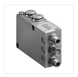
Bus coupler with driver Version 0 ... 50 °C Ambient temperature min./max. Operational voltage electronics 24 V DC -15% / +20% Electronics voltage tolerance 0,05 A Power consumption electronics Operating voltage, actuators 24 V DC Total current for actuators 3 A Protection class IP65 Number of solenoid coils max. 32 Max. power consumption per coil 0,1 mA Generic emission standard in accordance EN 61000-6-4 with norm
