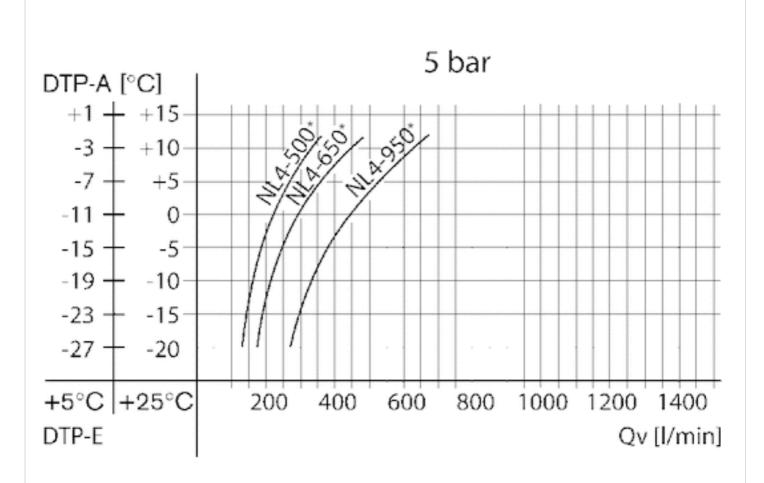
DTP-E: pressure dew point input DTP-A: pressure dew point output
