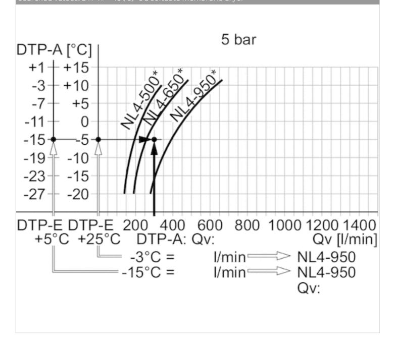
Result: membrane dryer series NL4-950 (with a Qn of 950 l/min), part no. R412007608
