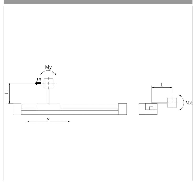
L indicates the distance between the mounting plate center and the center of mass of the attached parts.
