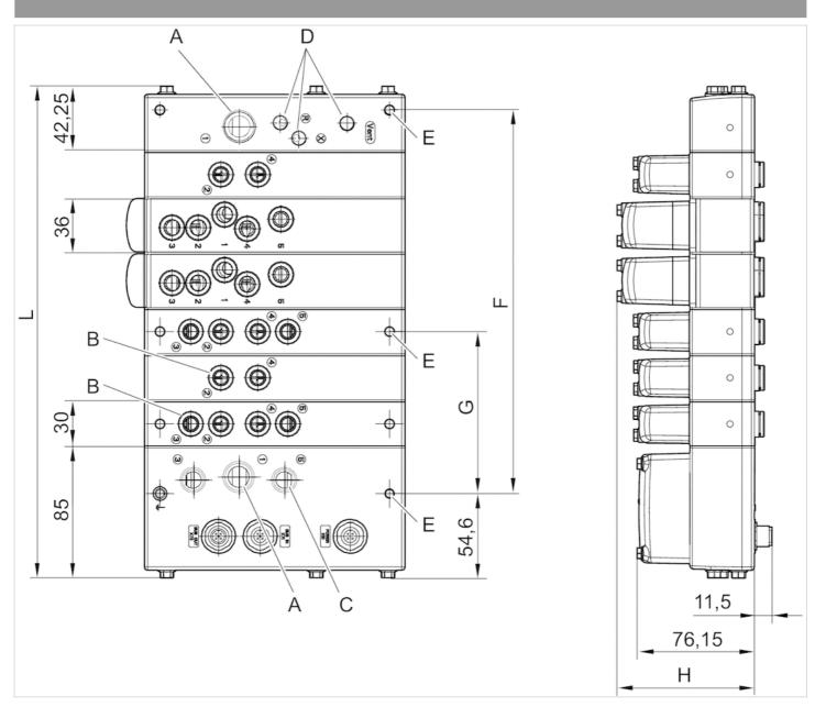
G = mounting on 4-ported subbase 0.60" + (number of 2-ported and 4-ported subbases) \* 1.18" + (number of 5-ported subbases) \* 1.42"G = mounting on 5-ported subbase 0.48" + (number of 2-ported and 4-ported subbases) \* 1.18" + (number of 5-ported subbases) \* 1.42"L = 5.01" + (number of 2-ported and 4-ported subbases) \* 1.18" + (number of 5-ported subbases) \* 1.42"H = 3.51" (IP69K version)
