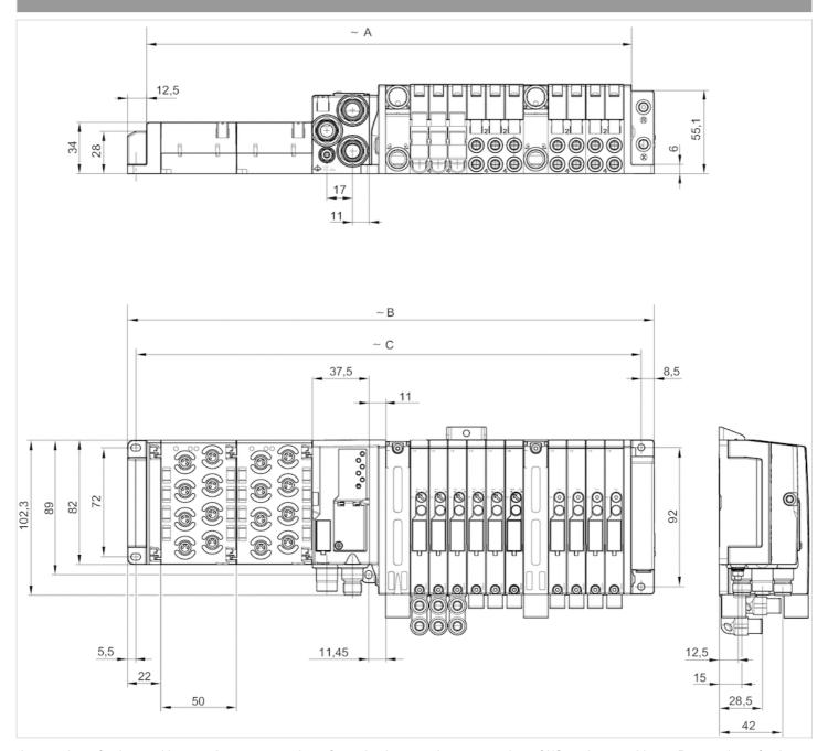
A = number of valve positions x 12.5 mm + number of supply plates x 16 mm + number of I/O x 50 mm + 63 mm B = number of valve positions x 12.5 mm + number of supply plates x 16 mm + number of I/O x 50 mm + 90.5 mm C = number of valve positions x 12.5 mm + number of supply plates x 16 mm + number of I/O x 50 mm + 76.5 mm
