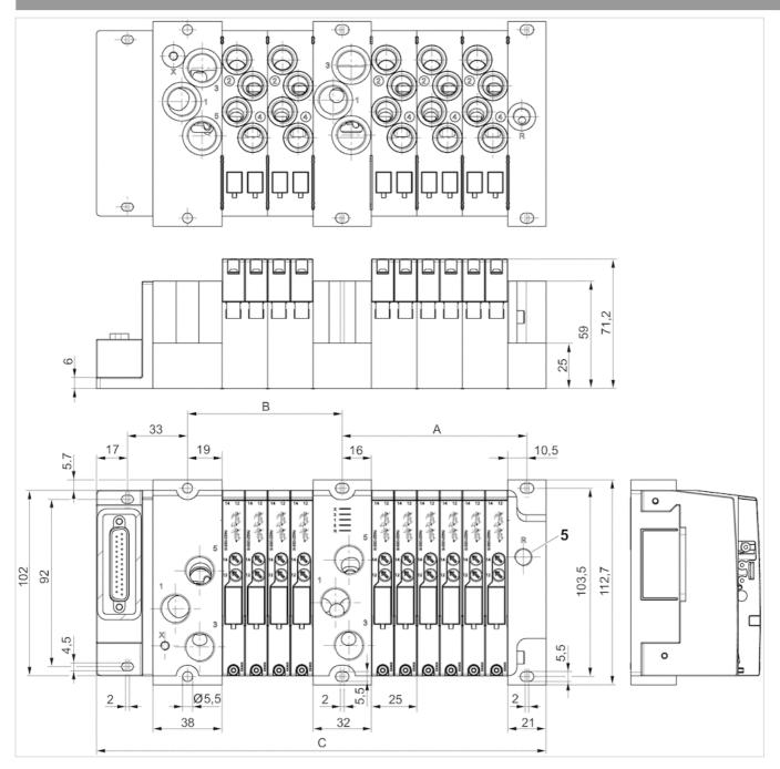
A = number of valve positions x 12.5 mm + 26.5 mmB = number of valve positions x 12.5 mm + 35 mm
