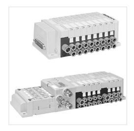
Mounting orientation Any Working pressure min./max. -0,95 ... 10 bar 3 ... 8 bar Control pressure min./max. -10 ... 60 °C Ambient temperature min./max. Medium temperature min./max. -10 ... 60 °C Compressed air Medium Max. particle size 40 µm Oil content of compressed air 0 ... 5 mg/m<sup>3</sup> Nominal flow Qn 300 l/min Number of valve positions max. 64 Protection class with connection IP65 24 V DC operating voltage
