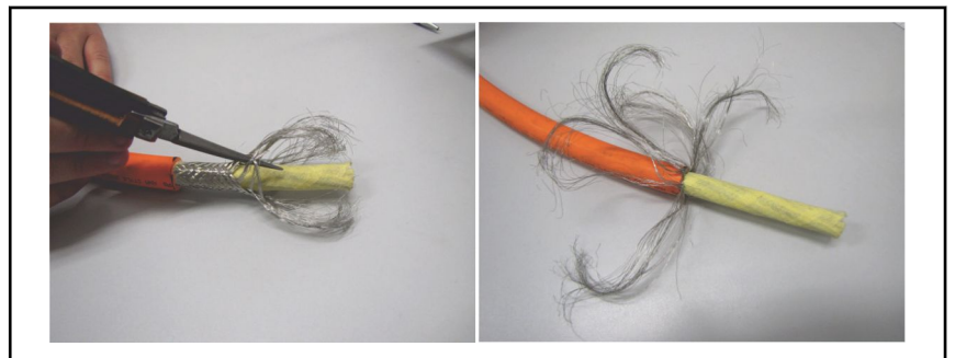
Fig. 8-5: Split the shield braid open
