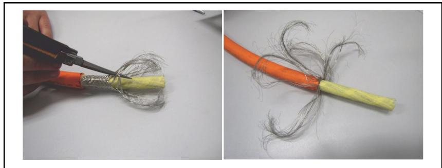
*Fig. 5-5: Split the shield braid open*
