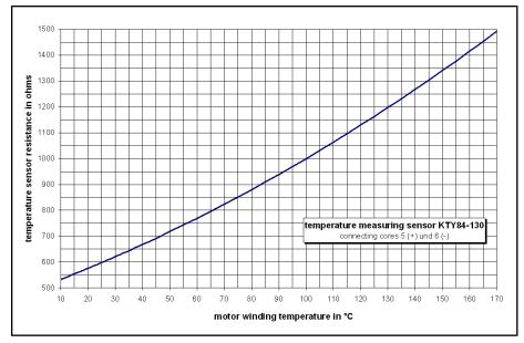
Fig.9-28: Characteristic of temperature measurement sensor KTY84-130 (PTC)
