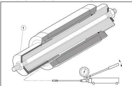
Assembly tools Fig.11-12: "Floating" of the rotor
