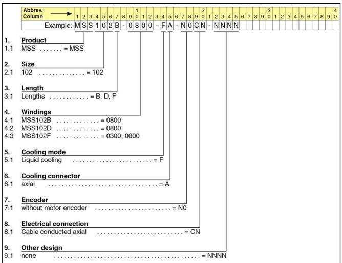
Fig.6-4: Type code MSS102
