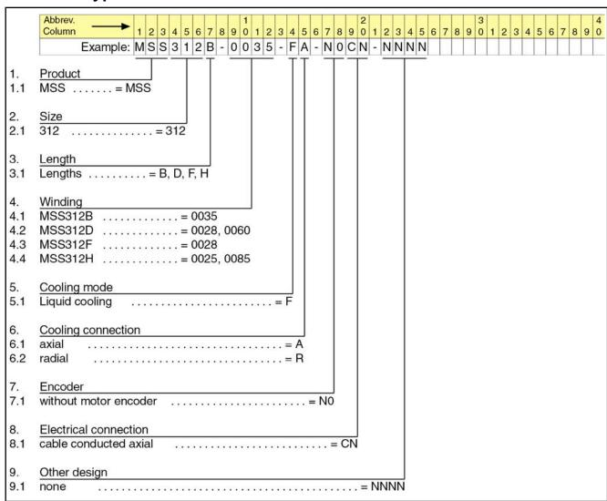
Fig.6-18: Type code MSS312
