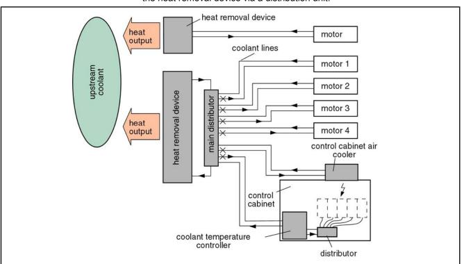
Fig.9-18: General arrangement of cooling systems with one and more drive components
