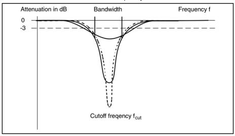
Fig. 12-7: Amplitude response of cutoff filter depending on bandwidth, qualitative
