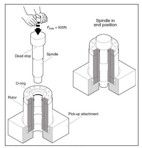
Assembling rotor and spindle
