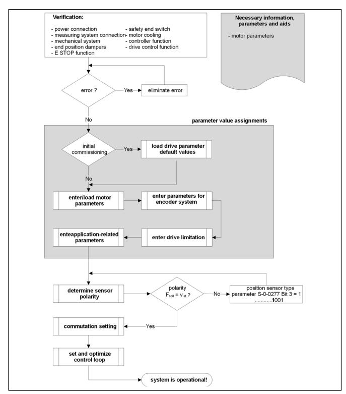
Fig. 12-1: General start-up procedure at synchronous-kit motors
