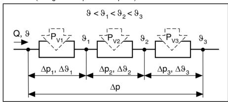
Fig.9-23: Series connection of liquid-cooled drive components
