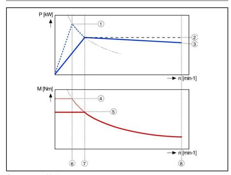
1 Maximum output Nominal power 2 3 Real power 4) Maximum torque (5) Nominal torque 6 Speed at Mmax 7 Nominal speed Maximum speed 8
