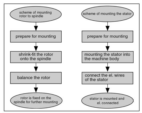
Fig. 11-1: Procedure for assembling the rotor and the stator
