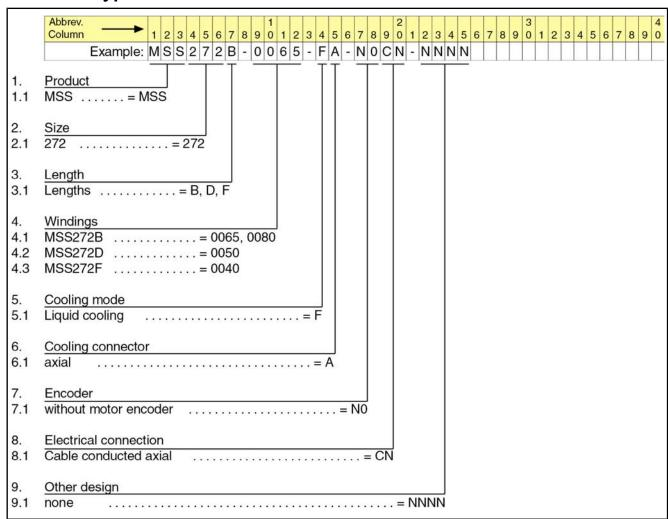
Fig.6-16: Type code MSS272
