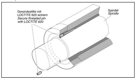
Fig. 11-11: Sealing the pressure oil connections
