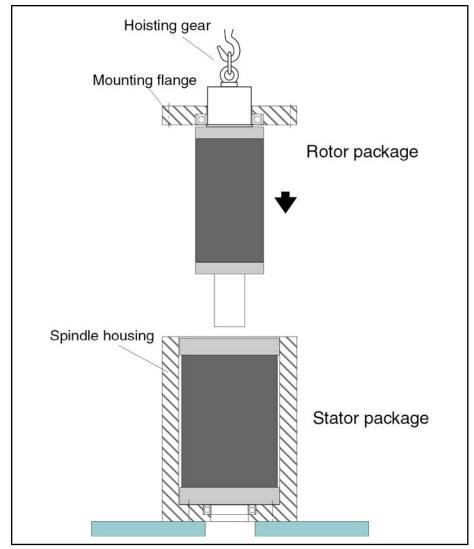
Fig. 11-22: Motor spindle assembly
