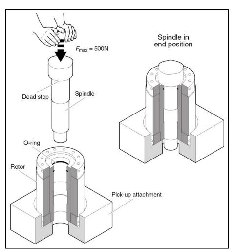
Fig. 11-7: Assembling rotor and spindle
