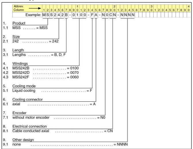
Fig.6-14: Type code MSS242
