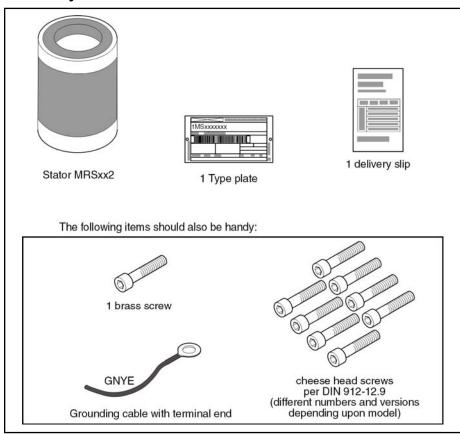
Fig.11-18: Scope of delivery of the stator and additional materials
