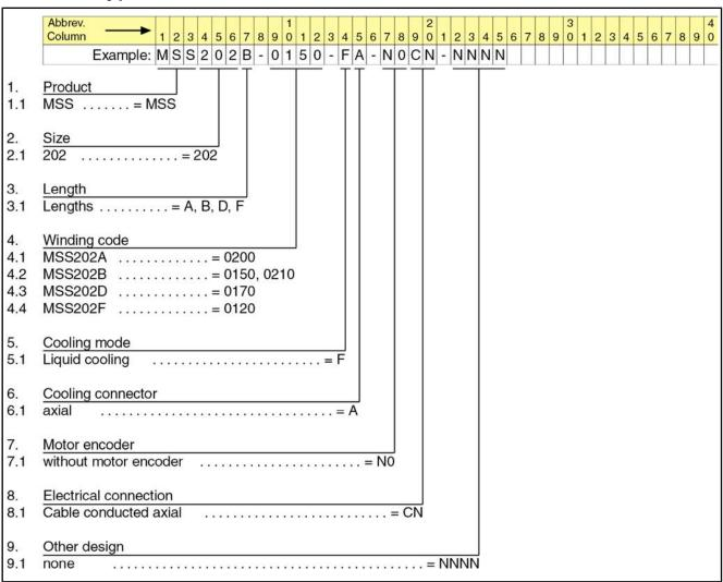
Fig.6-12: Type code MSS202
