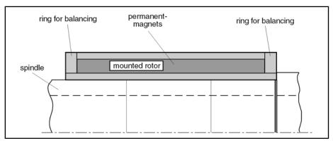
Fig.9-30: Rotor design 1N - smooth shaft
