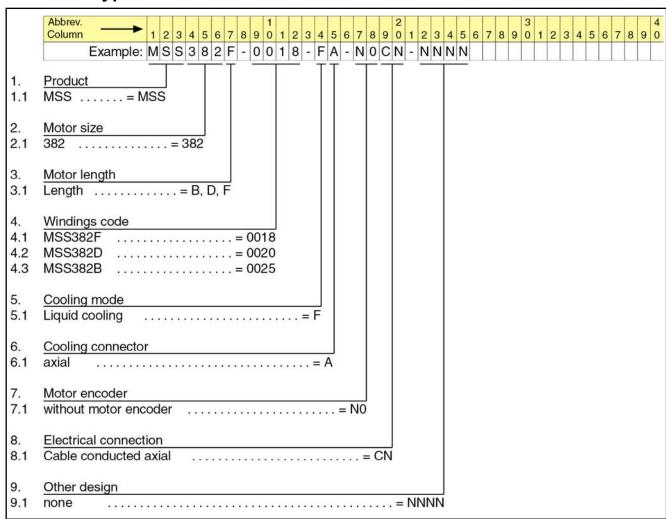
Fig.6-20: Type code MSS382
