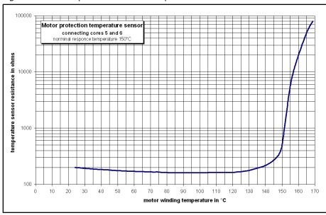
Fig.9-27: Characteristic of motor protection sensors (PTC)
