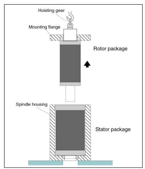
Fig.11-25: Dismantling the motor spindle
