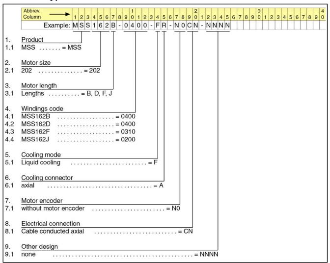
Fig.6-8: Type code MSS162
