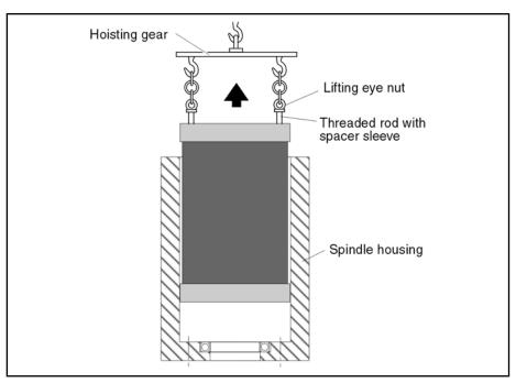
Fig. 11-21: Removing the stator from the spindle housing
