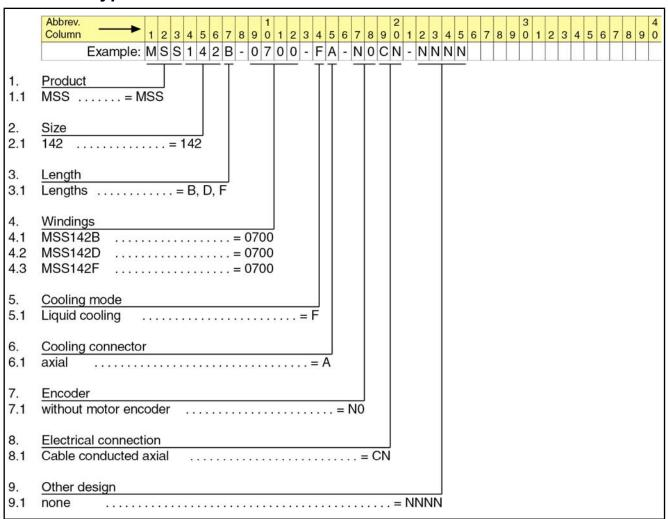
Fig.6-6: Type code MSS142
