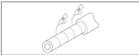
Fig. 11-6: Preparing the spindle for assembly
