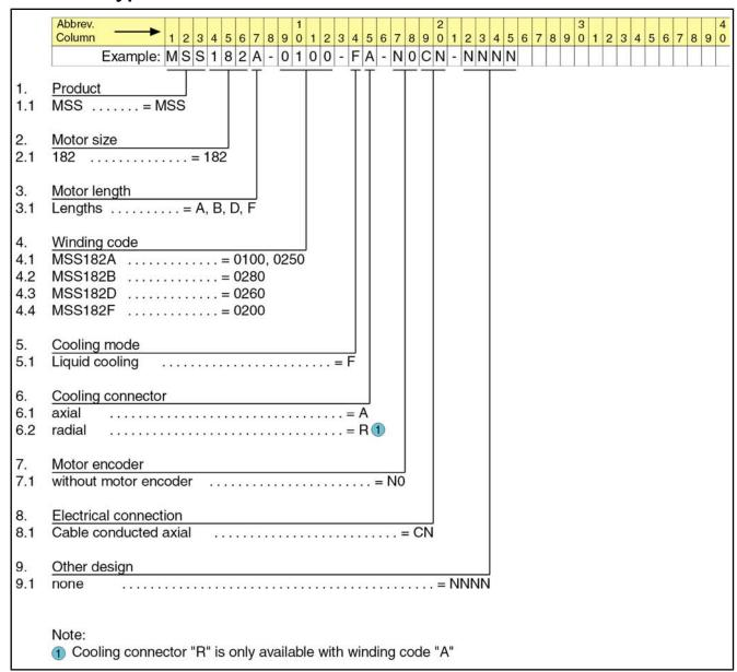
Fig.6-10: Type code MSS182
