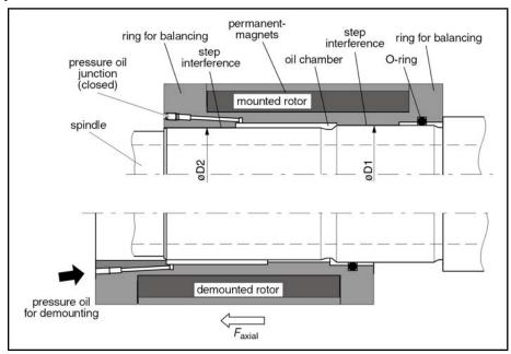
Fig.9-31: Rotor installation and functional principle of the step interference fit
