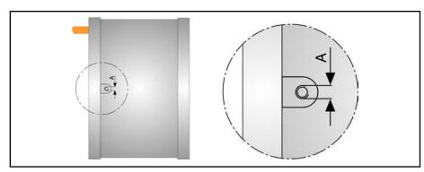
Fig.8-14: Radial cooling connection
