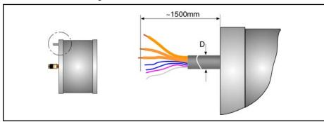
D Diameter cable harness Fig.8-1: IndraDyn H cable harness
