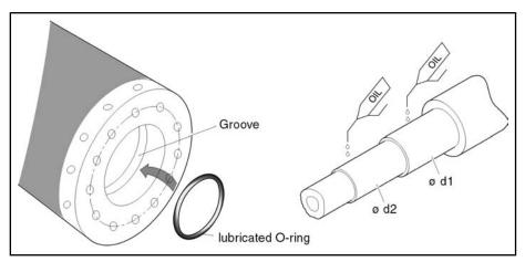
Fig. 11-9: Preparing the rotor and the spindle for assembly
