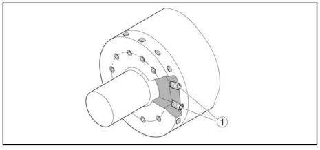
Securing screws using Loctite 620Fig. 11-14: Balancing by inserting threaded pins
