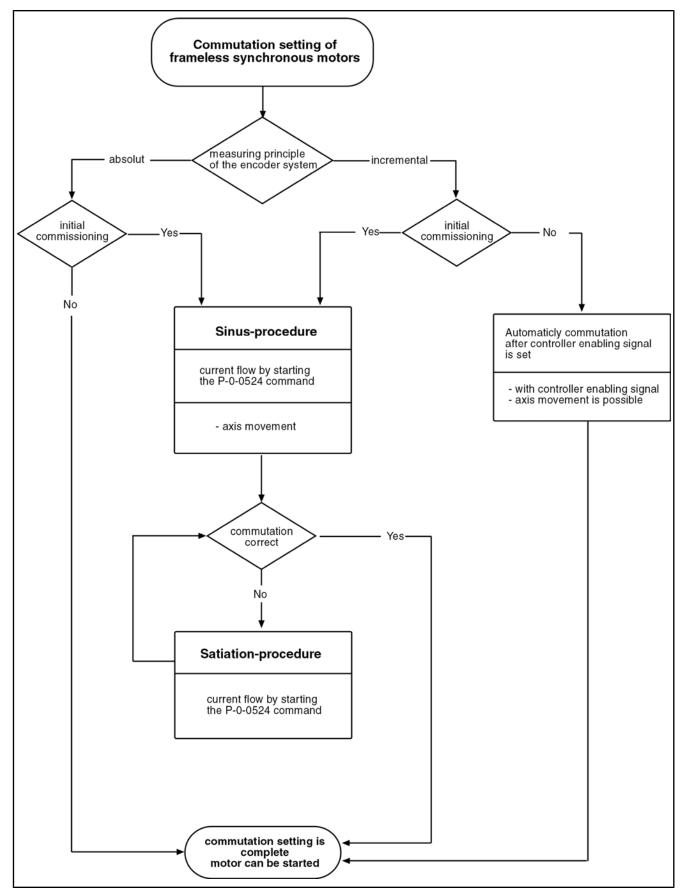
Fig. 12-5: Commutation adjustment method for synchronous kit motors
