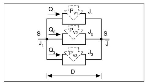
Fig.9-21: Parallel connection of liquid-cooled drive components
