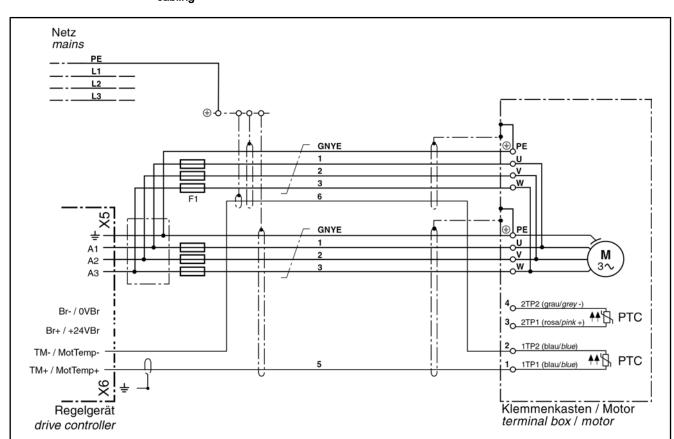
Fig.8-8: Connection diagram double cabling
