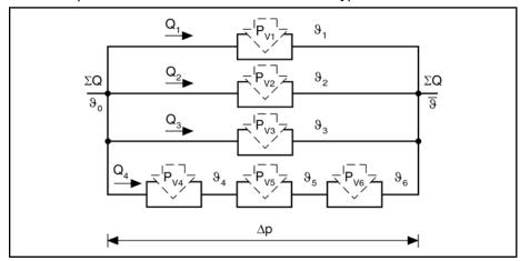
Fig.9-25: Combination of series and parallel connection
