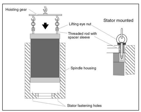
Fig. 11-19: Installing the stator into the spindle housing
