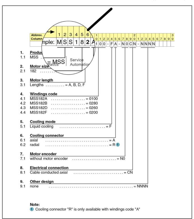
Fig.6-2: IndraDyn H type code example MSS
