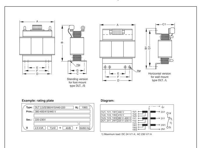
Dimensions and technical data for three phase isolation transformer with U  $_{\rm Sec}$  = 220-230 V;  $\rm U_{pri}$  = 380-400 V, 415 V, 440 V, 460 V, 500 V, f = 50/60 Hz
