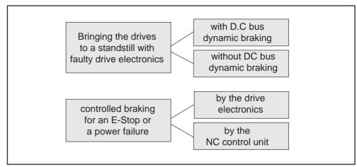
Figure 4.1: Differentiating features of the power circuits
