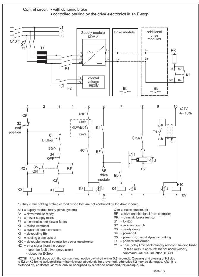
Figure 4.4: Control circuits without soft-start resistor with dynamic braking
