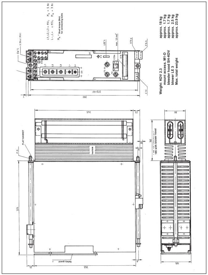
Figure 7.1: Dimensional data for the KDV 2.3 supply module
