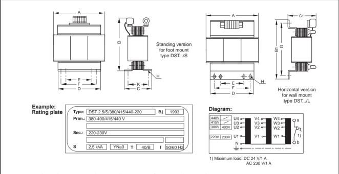
Dimensions and technical data for 3-phase AC autotransformer with  $\rm U_{sec}$  = 220-230 V;  $\rm U_{pri}$  = 380-400 V, 415 V, 440 V, 460 V, 500 V, f = 50/60 Hz
