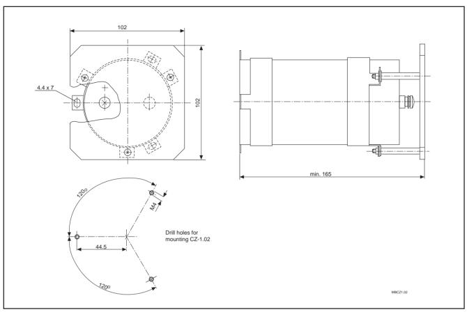
Figure 7.4: Dimensional data for the CZ 1.02 additional capacitor
