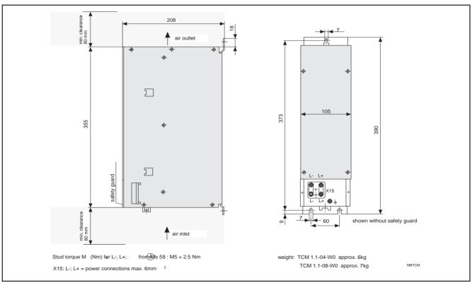
Figure 7.5: Dimensional data for the TCM additional capacitor module
