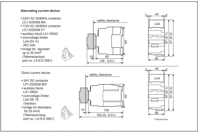
Figure 7.7: Dimensional data for dynamic brake contactor
