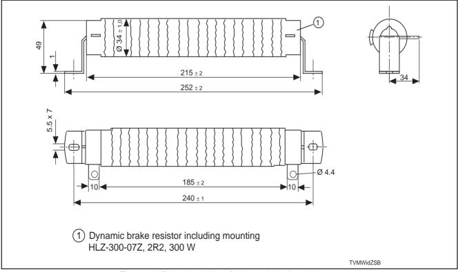
Figure 7.8: Dimensional data for dynamic brake resistor
