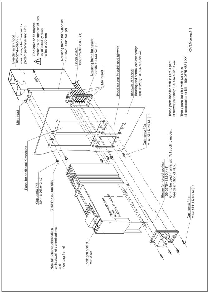
Figure 3.13: Mounting the KDV 2.3 into the control cabinet
