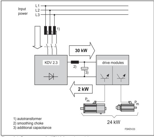
Figure 2.1: Power range of a KDV 2.3 supply module
