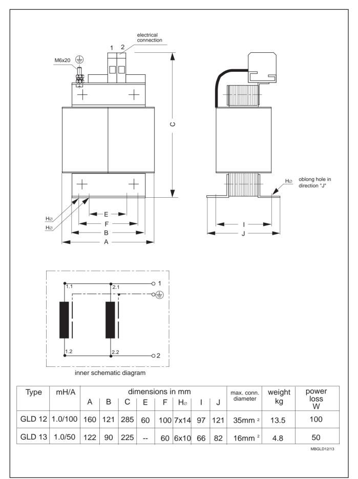
Figure 7.6: GLD 12/13 smoothing choke - dimensional data
