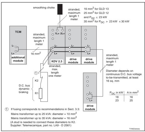
Figure 3.7: DC bus wiring
