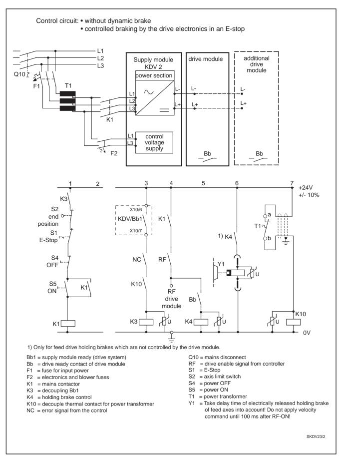
Figure 4.5: Control circuits for KDV 2.3 without dynamic braking
