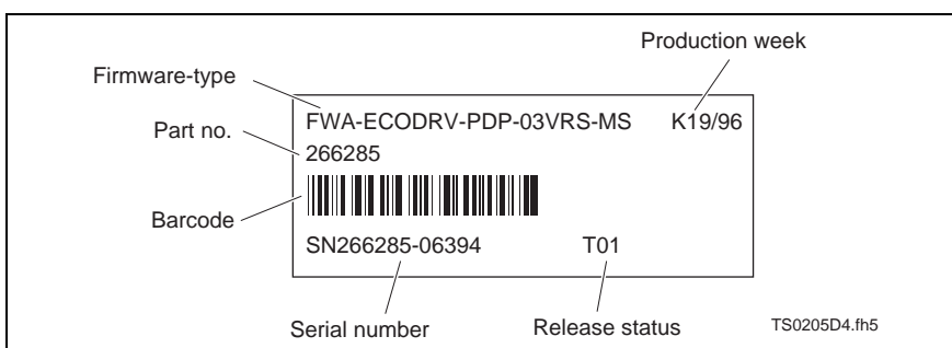
Fig. 4-11: Rating plate firmware
