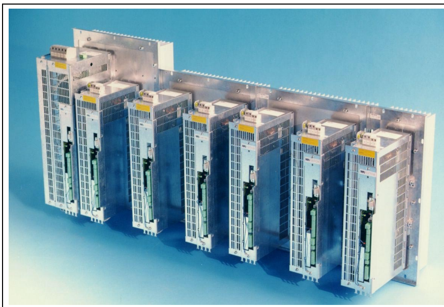
Fig. 2-2: Project with units from the REFUreduc series: Multi-motor drive with degree of protection IP 54 (NEMA 12) through connection mounting with textile heatsinks and mounting frames
