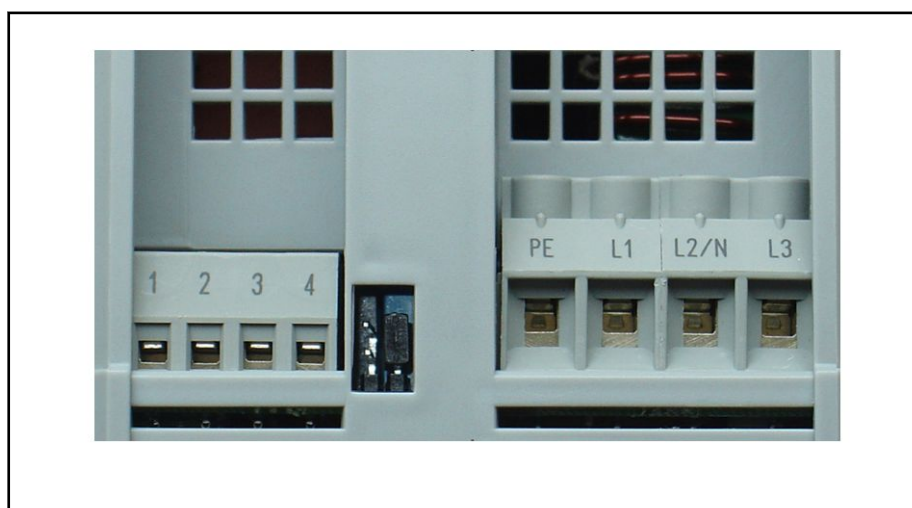
Fig.5-6: Mains Input Jumper in Position "2"
