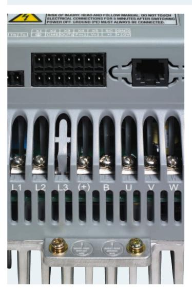
The terminal side: plug-in terminal for peripherals
