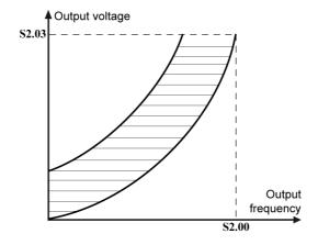
Fig.8-19: Square V/F curve auto torque boost
