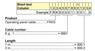
Fig.17-6: Operating panel cable type coding
