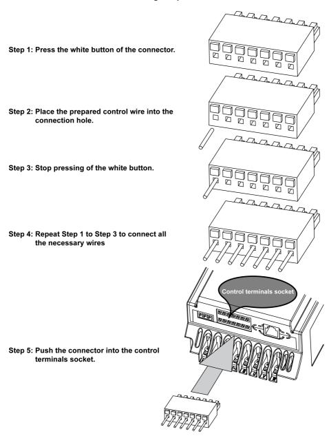
Fig.5-16: Control Circuit Wiring Steps 42/235
