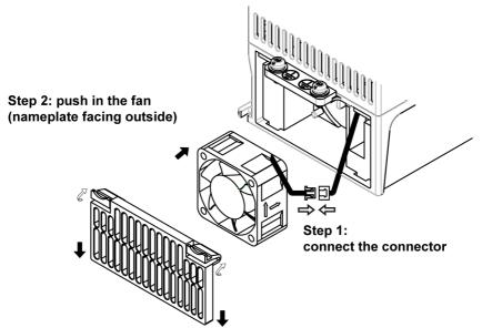
Step 3: insert the cover into the lower slots, rotate the cover and push the buckles into the upper slots
