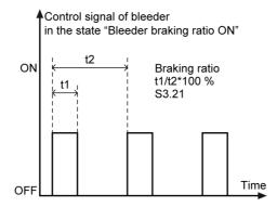
Fig.8-41: Switching pattern\_Maximum duty cycle
