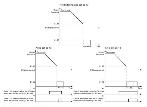
Fig.8-8: Stopping DC braking
