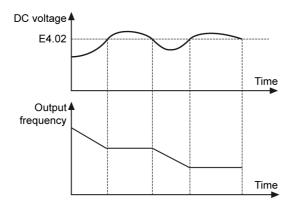
Fig.8-43: Stall overvoltage prevention level\_during deceleration
