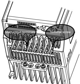
Step 1: Loosen terminal screws.
