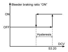
Fig.8-42: Switching pattern\_Hysteresis voltage
