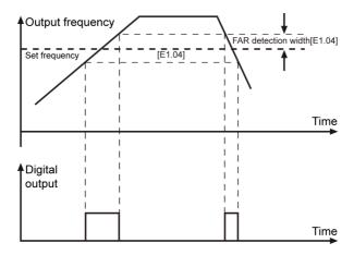
Fig.8-37: Frequency arriving at detection width
