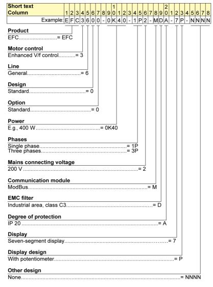
Fig.17-1: EFC 3600 type coding
