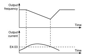
Fig.8-45: Stall overcurrent prevention level\_at constant speed
