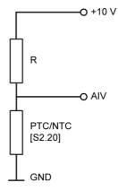
Fig.8-21: Protection with temperature sensor
