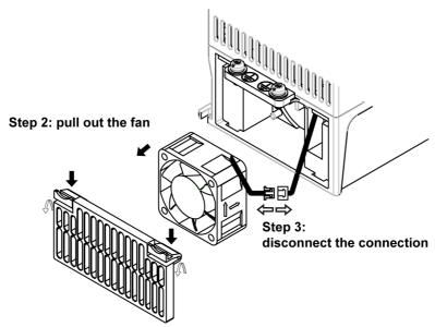
Step 1: press the two plate buckles and rotate to remove the plate
