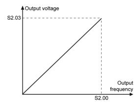
Fig.8-9: Linear curve
