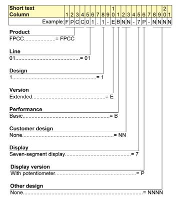
Fig.17-2: Operating panel type coding
