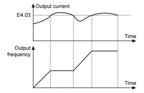
Fig.8-44: Stall overcurrent prevention level\_during acceleration
