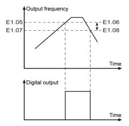
Fig.8-38: Frequency detection level
