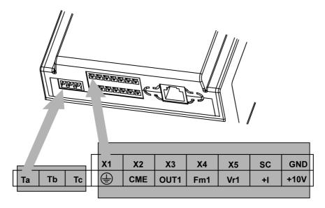
Fig.5-12: Control circuit terminals
