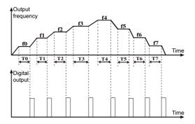
Fig.8-34: Simple PLC phase completion indication
