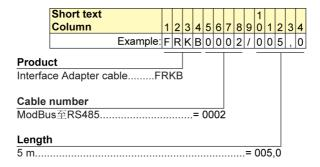
Fig.17-5: Interface adapter cable type coding
