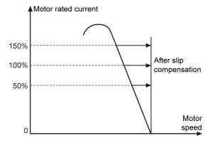
Fig.8-14: Slip frequency compensation
