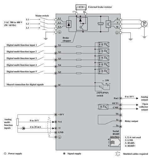
Fig.5-6: Block diagram (3AC)
