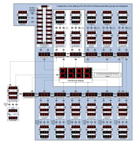
Fig.6-5: Example of operating panel operation
