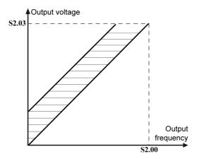
Fig.8-18: Linear V/F curve auto torque boost
