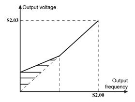
Fig.8-16: Linear V/F curve manual torque increase
