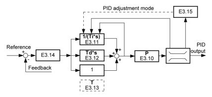
Fig.8-40: PID control principle
