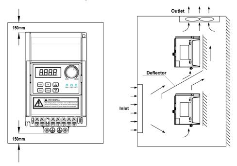
Fig.5-3: EFC 3600 mounting
