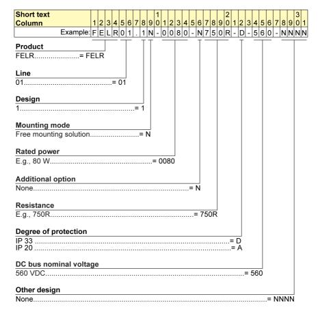
Fig.17-3: Braking resistor type coding
