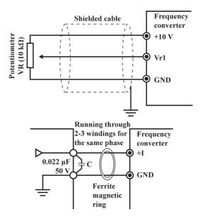
Fig.5-15: Analog Input Terminals (+10 V, Vr1, GND,+I)
