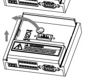
Fig.14-1: Operating panel removal
