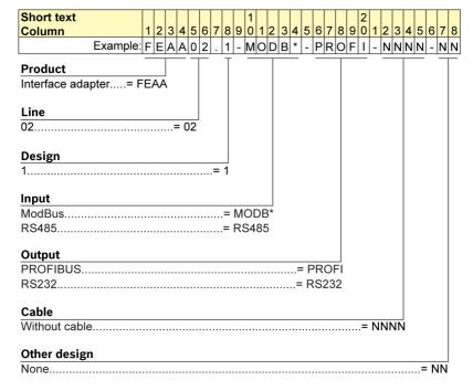
Fig.17-4: Interface adapter type coding
