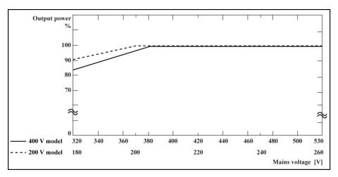
Fig.10-1: Derating and mains voltage
