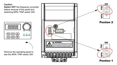
Fig.5-13: NPN / PNP Switch SW for the Digital Inputs
