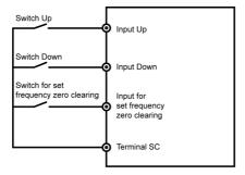
Fig.8-26: External terminals Up / Down settings
