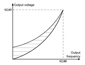
Fig.8-17: Square V/F curve manual torque increase
