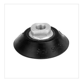
Ambient temperature min./max.  $-10 \dots 70 \,^{\circ}\text{C}$  Hardness according to standard  $60 \pm 5 \, \text{Shore A}$  Abrasion value according to DIN 535 16  $105 \, \text{mm}^{3}$  Weight See table below
