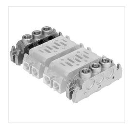
Standards ISO 5599-1 Compressed air connection according to ISO 5599-1 Working pressure min./max. -1 ... 16 bar -20 ... 70 °C Ambient temperature min./max. -20 ... 70 °C Medium temperature min./max. Medium Compressed air Direction of pneumatic port (1) Both directions possible Direction of pneumatic port (3,5) Both directions possible Exhaust (3,5) uncollected exhaust Exhaust type Ports separated Weight
