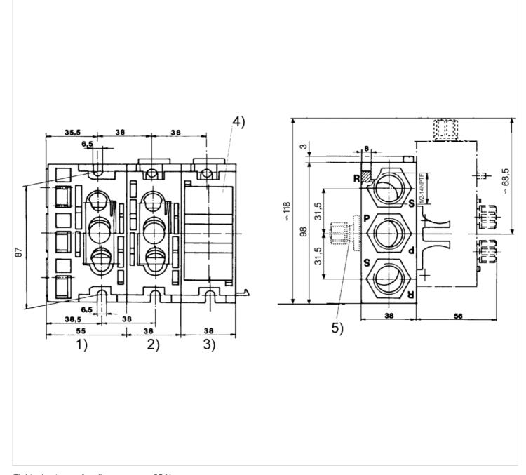
Tightening torque for all screws max. 35 Nm
