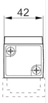
1) Tightening torque for mounting screws: 2.7  $\pm$  0.3 Nm Base plate not included in the scope of delivery
