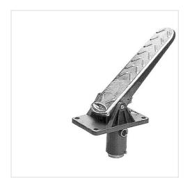
Туре Poppet valve Working pressure min./max. 0.1 ... 10 bar Adjustment range min./max. See table below -25 ... 70 °C Ambient temperature min./max. Medium temperature min./max. -25 ... 70 °C Medium Compressed air Nominal flow Qn 900 l/min Hysteresis 0.15 bar Weight 1.5 kg
