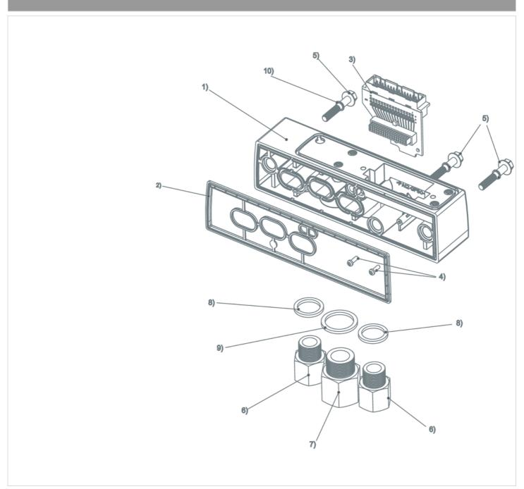
1) Connection piece 2) Seal 3) Circuit board connection piece 4) Screws 5) Screw M5x30 For additional inch-versions: 6) Adapter G 1/8 - NPTF 1/8 7) Adapter G 3/8 8) Seal for connecting fittings 9) Seal
