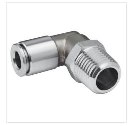
Working pressure min./max. Ambient temperature min./max. Weight per piece -0,95 ... 16 bar -20 ... 150 °C See table below
