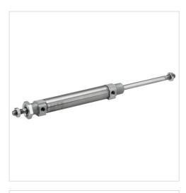
Standards ISO 6432 Certificates ATEX optional Compressed air connection Internal thread Working pressure min./max. 1 ... 10 bar -25 ... 80 °C Ambient temperature min./max. Medium temperature min./max. -25 ... 80 °C Medium Compressed air 50 µm Max. particle size 0 ... 5 mg/m<sup>3</sup>
