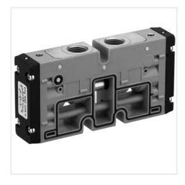
Туре Spool valve, positive overlapping Activation pneumatically Pilot External Sealing principle Soft sealing Plate principle Blocking principle 1300 l/min Flow rate value Qn -0,9 ... 10 bar Working pressure min./max. 3 ... 10 bar Control pressure min./max. -10 ... 50 °C Ambient temperature min./max. -10 ... 50 °C Medium temperature min./max. Max. particle size 5 µm
