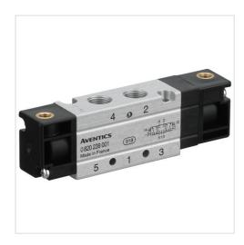
Type Spool valve, positive overlapping Activation pneumatically Pilot External Sealing principle Soft sealing Working pressure min./max. -0,9 ... 10 bar Control pressure min./max. 2,2 ... 10 bar 0 ... 80 °C Ambient temperature min./max. 0 ... 80 °C Medium temperature min./max. Medium Compressed air
