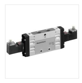
Туре Spool valve, positive overlapping Activation Electrically Sealing principle Soft sealing See table below Working pressure min./max. Control pressure min./max. 3 ... 10 bar -10 ... 50 °C Ambient temperature min./max. -10 ... 50 °C Medium temperature min./max. Medium Compressed air Max. particle size 5 µm
