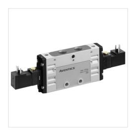
Spool valve, positive overlapping Туре Activation Electrically Sealing principle Soft sealing See table below Working pressure min./max. Control pressure min./max. 3 ... 10 bar -10 ... 50 °C Ambient temperature min./max. -10 ... 50 °C Medium temperature min./max. Medium Compressed air Max. particle size 5 µm Oil content of compressed air 0 ... 5 mg/m<sup>3</sup>
