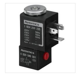
Poppet valve Type Activation Electrically Sealing principle Soft sealing Working pressure min./max. See table below -10 ... 50 °C Ambient temperature min./max. -10 ... 50 °C Medium temperature min./max. Medium Compressed air Max. particle size 5 µm
